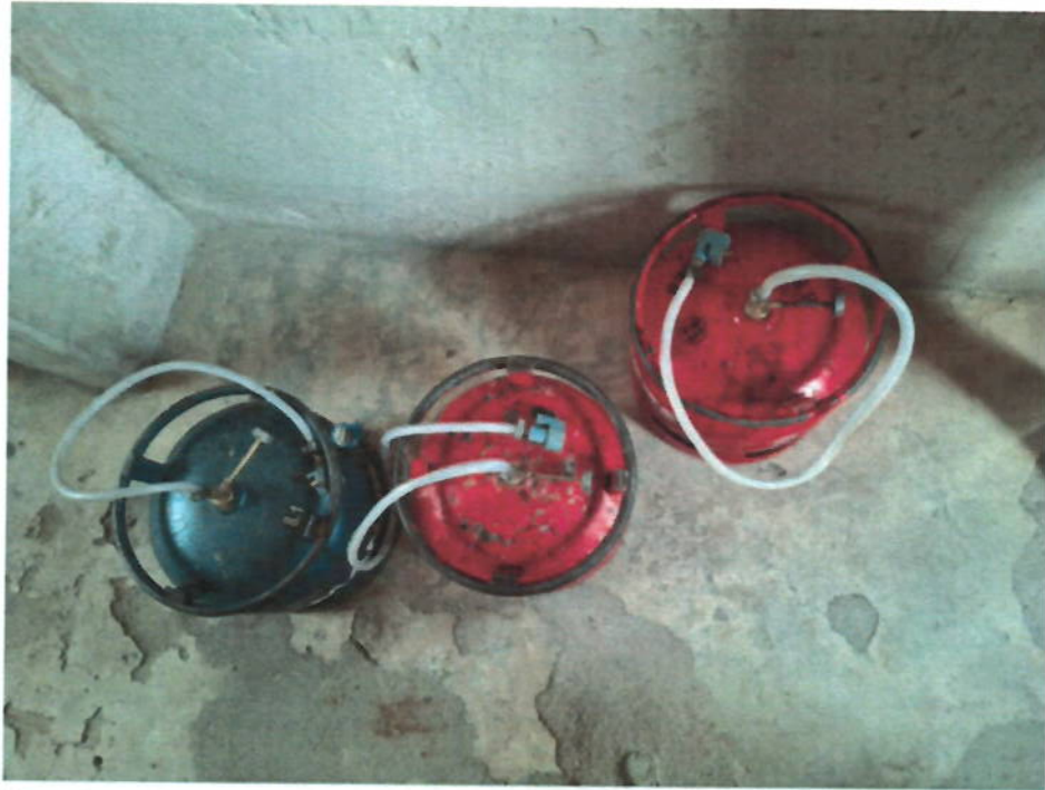
Photo 8: Devices used in decanting and refilling of cylinders seized by The Fire and Rescue Services Force
